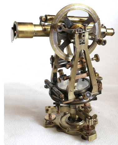
A theodolite of the transit type with six-inch circles, manufactured in Britain around 1910 by Troughton & Simms in London.
